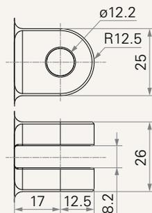
C = Aluminum casting, U clevis, slot 8.2, depth 17.0, hole 10.2, with T-bushing
