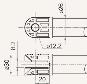
5 = Punched hole on inner tube, without slot, hole 10.2, with plastic bush
