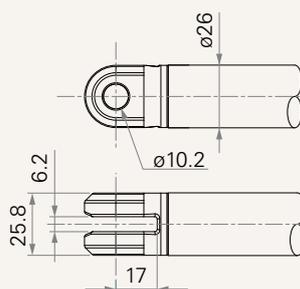
8 = Aluminum casting, U clevis, width 6.2, depth 17.0, hole 12.2
