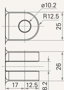
3 = Aluminum casting, U clevis, slot 8.2, depth 17.0, hole 12.2
