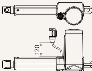
R = Extension cable, preset on motor cover (cable length 50mm)
