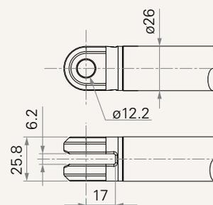
9 = Aluminum casting, U clevis, width 6.2, depth 17.0, hole 10.2, with T-bushing
