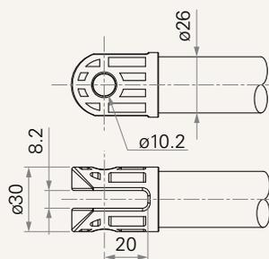
4 = Plastic, U clevis, width 8.2, depth 20.0, hole 12.2, for push < 4000N and pull < 2500N
