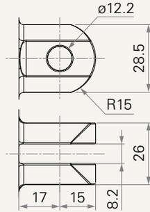
4 = Aluminum casting, U clevis, width 8.2, depth 17.0, hole 10.2 (for push ≥ 4000N)
