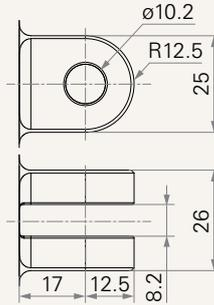
5 = Aluminum casting, U clevis, width 8.2, depth 17.0, hole 12.2 (for push ≥ 4000N)
