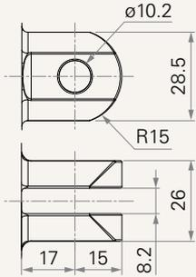
3 = Plastic, U clevis, width 8.2, depth 17.0, hole 12.2 (for push < 4000N)
