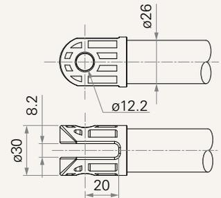
5 = Punched hole on inner Aluminum tube, without slot, hole 10.2, plastic bush
