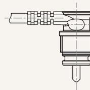
C = Y cable (for direct cut system, water proof, anti pull)
